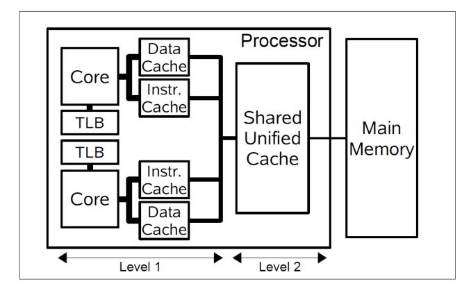
OpenMP can be applied to a multicore processor with shared memory.
