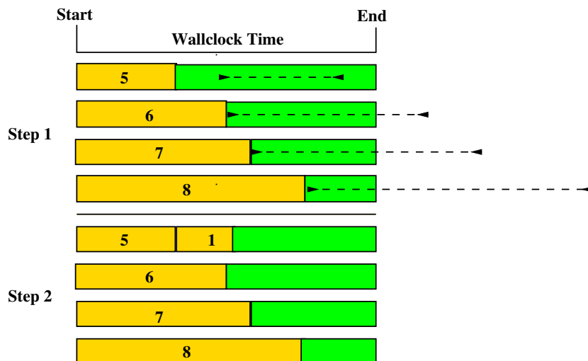
Figure 2: A successful job scenario. Step 1 shows the first set of tasks to be executed. The green boxes indicate the actual walltime remaining. The dashed lines indicates the maximum walltime to allow for the next job, based on what has completed so far.
