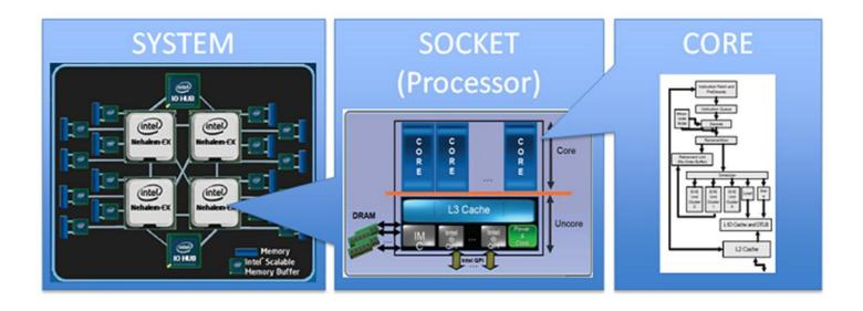
> 4 cores/processor \* 4 processors = 16 total cores
